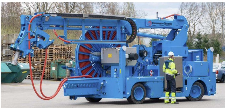
Ferries and ro-pax vessels – Example of a mobile CMS with 1 power cable – Gdynia, Poland Mobile CMSs are much more expensive to purchase and operate.
