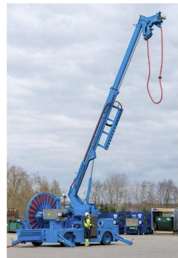
Ferries and ro-pax vessels – Example of a mobile CMS with 1 power cable – Gdynia, Poland Mobile CMSs are much more expensive to purchase and operate.
