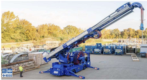
Cruises – Examples of mobile CMS with 7 cables, including 4 power cables – Southampton and Norway
