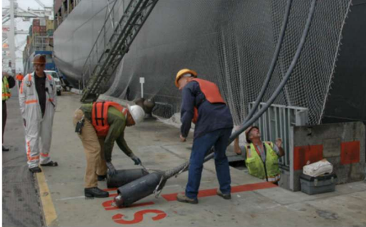
Sockets connected directly to the PIT Container ship with two cables connected on the quay
