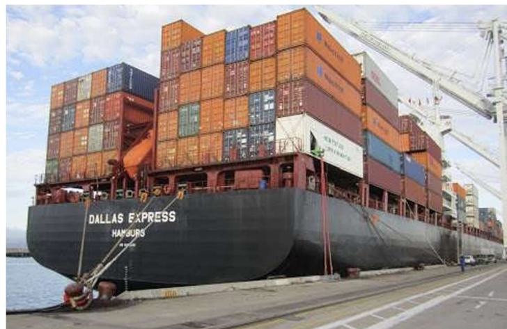
AMP connection container on starboard side with direct connection to the quayside PIT (without CMS Cable Management System)
